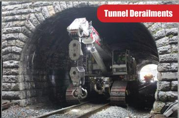
The Dynamic envelope is very advantageous in tunnels. The 200 RS with its lifting ability in a confined space coupled with a forward or backward positionable recovery winch is the most efficient piece of equipment in the industry when it comes to tunnels.
