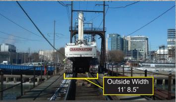
Single main or double main. Either location is easily accessible with adjustable, padded tracks extend from an outside width of 11' 8" to a maximum width of 17' 4". The padded tracks help to minimize impact, while the addition of swamp mats increases the protection. The ability to vary track width independently also maximizes lifting capability by allowing the crane to shift its position side to side while leaving the tracks stationary.
